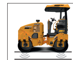
COMPACTION FORCE Optimized setting amplitude, frequency and optimum distribution of weight helps in achieving high compaction
