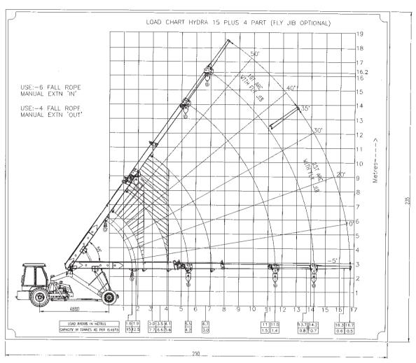
Rated loads are calculated for operation on leveled surface.
