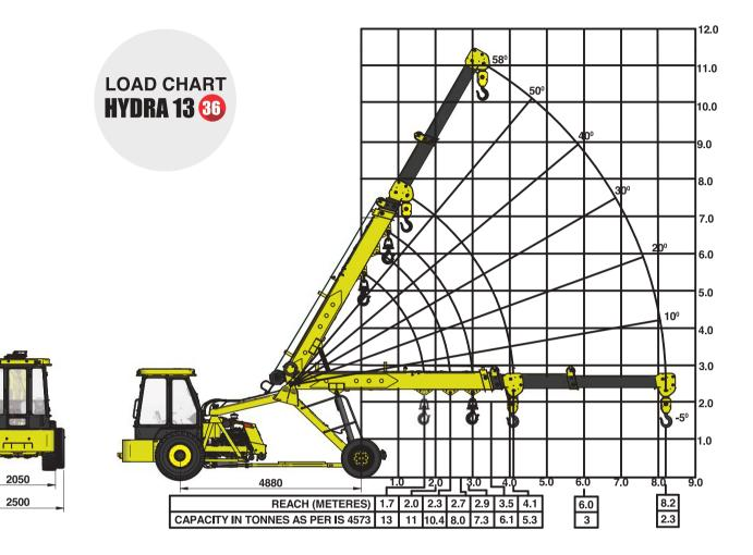
Rated loads are calculated for operation on leveled surface.
